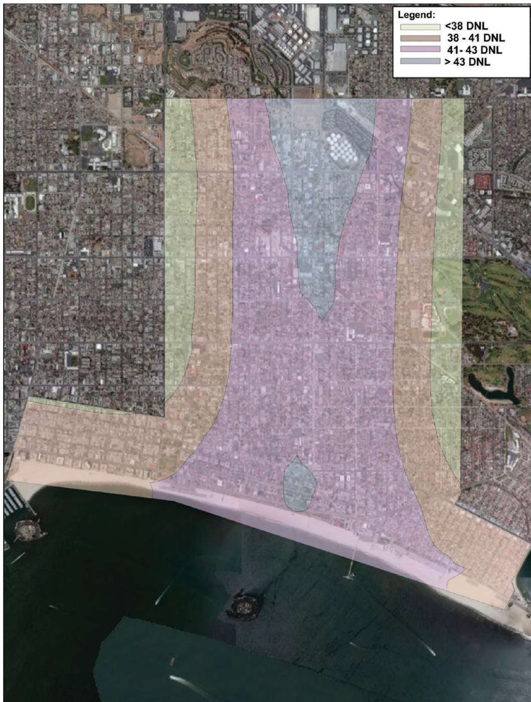
Figure 4-11. Preliminary helicopter-only noise exposure bands in vicinity of helicopter flight tracks at LGB.
